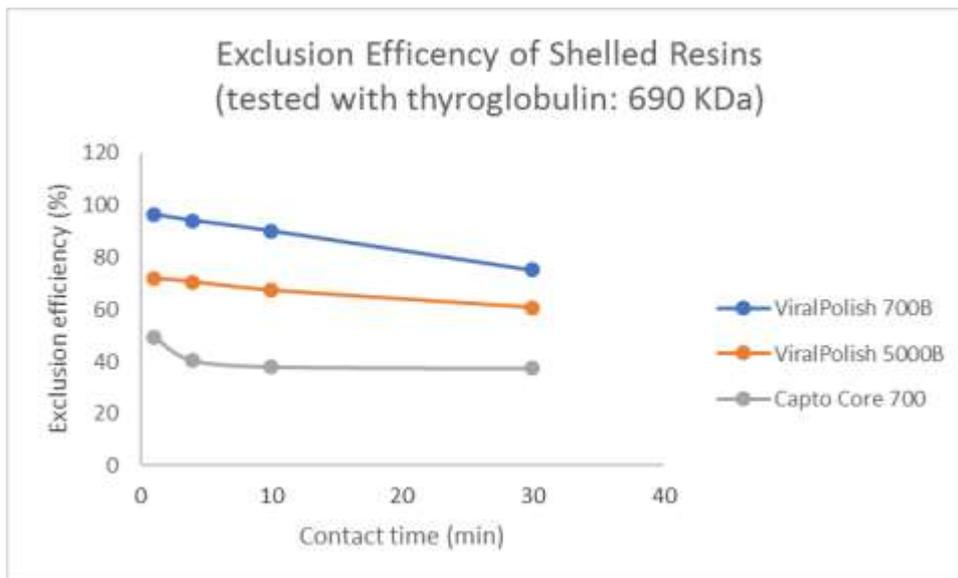
**Figure 3:** Size-exclusion effectiveness of SepFast DUO type of media is further demonstrated using shelled media having mixed-mode ligands inside. ViralPolish range of media has the same bead structure as SepFast DUO but the ligand inside is mixed-mode ligand tolerating high salt, designed to bind all smaller size impurities to provide a flow-through 'clean up' step.
