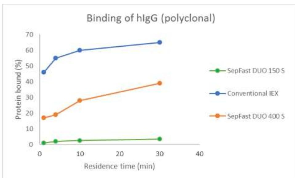
**Figure 2:** Comparison of the binding performance of conventional porous ion-exchange medium to SepFast DUO media having different size-exclusion shells. Note the very efficient exclusion of human immunoglobulin molecule (around 150 KDa) from the active binding core of SepFast 150 S.
