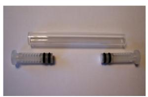
The **column body** (i.e. the tube) is made of acrylic. It has an appearance similar to a glass tube, i.e. clear and transparent.
